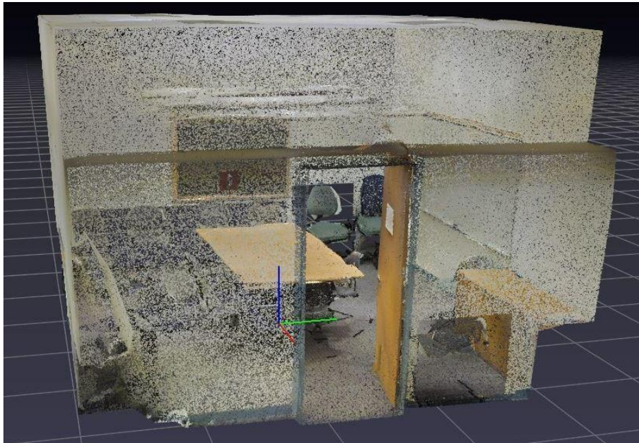
Raw point cloud of a meeting room
